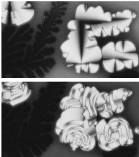
FIGURE 4 Liquid-crystalline textures shown on cooling by 3b at 77°C ( top ) and at 18°C ( bottom ). Crossed polarizers microscope.
